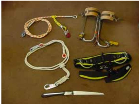
3. Steel core flip line with, locking snap on one end, and steel core prusik with locking snap, meeting ANSI A10.14 type 1 standards. Minimum length 16'
